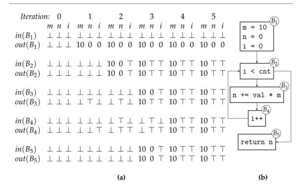
**Figure 2.11:** This figure shows the facts calculated for all nodes in our example program. Part (a) shows the *in* and *out* facts associated with each node. Part (b) reproduces the control-flow graph for our program. After 5 iterations the facts reach a fixed point (i.e., they stop changing) and we can see that  $in(B_3)$  shows that *m* is always 10, proving we can rewrite the multiplication safely.
