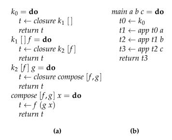
**Figure 4.4:** Part 4.4 (a) shows a rewritten version of *compose* that makes closure allocation explicit; Part 4.4 (b) gives a program that evaluates *compose a b c*. Note that these programs produce monadic values rather than pure values.
