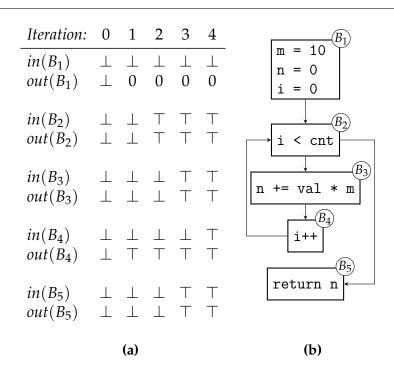
**Figure 2.8:** This figure shows the values for *i* calculated by all nodes in our example program. Part (a) shows the *in* and *out* facts associated with each node, for variable *i*. Part (b) reproduces the control-flow graph for our program. After 4 iterations the facts reach a fixed point (i.e., they stop changing).
