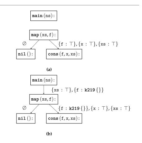
**Figure 5.15:** Facts that flow between blocks in our example program. Part (a) shows the CFG before we rewrite main; Part (b) shows the CFG afterwards. The facts from main only flow to the rest of the CFG after rewriting.
