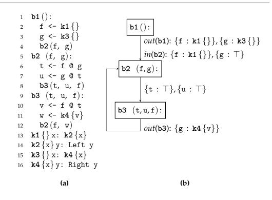
Figure 5.18: A MIL program with looping control-flow.
