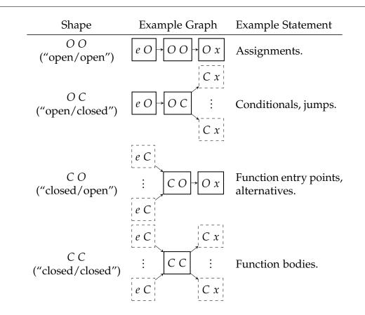
**Figure 3.2:** This table shows the four possible block shapes. Each row gives example statements and a representative CFG using a block of the given shape. Dashed lines indicate optional blocks. Solid lines show required blocks.
