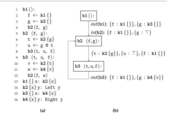
**Figure 5.19:** Our rewritten MIL program, showing that we correctly uncurried f @ g in b2; g @ t remains unchanged.
