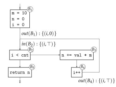
**Figure 2.4:** Our program, annotated with facts partway through the analysis. Notice that  $out(B_1)$  and  $out(B_4)$  give differing values to *i*. We use a *meet operator* when combining these two values while calculating  $in(B_2)$ .
